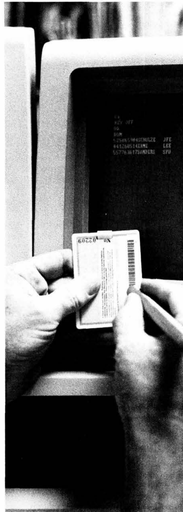
BADGE BAR CODE DISPLAYED — A light-pen reads the bar code on the back of an employee's badge. The computer displays and records the employee's social security number, name, initials, and clearance status, giving security inspectors a quick and accurate census of employees and visitors in a controlled area.
